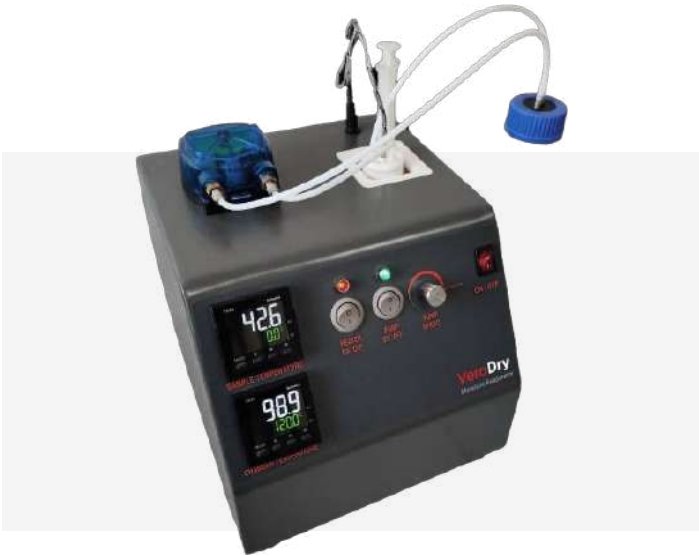
Figure 1: VeroDry Closed-Loop Evaporator
